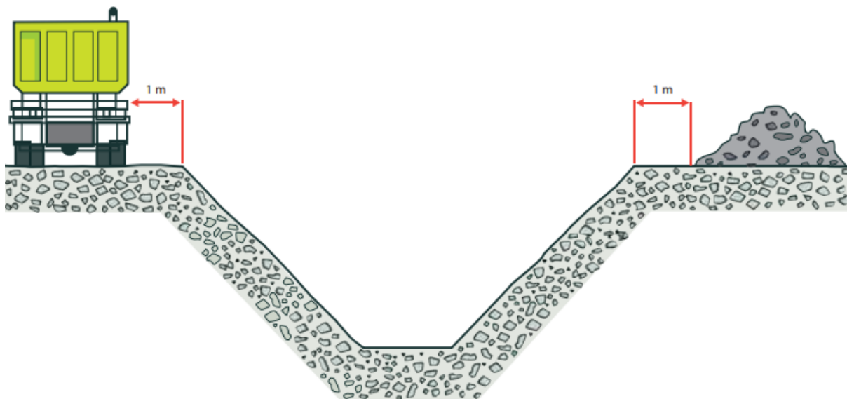
Figure 4 - Example of battering
